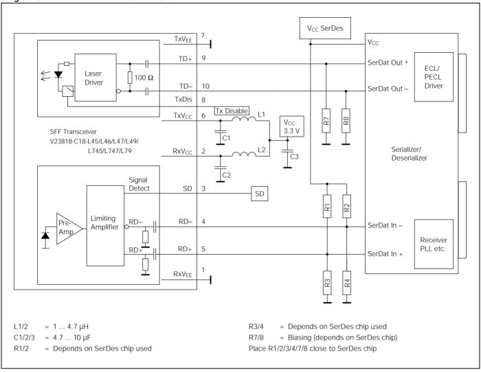
Values of R1/2/3/4 may vary as long as proper 50  $\Omega$  termination to  $V_{FF}$  or 100  $\Omega$  differential is provided. The power supply filter-
