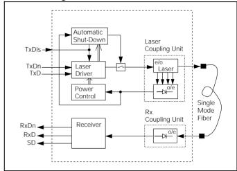
The receiver component converts the optical serial data into PECL compatible electrical data (RD+ and RD-). The Signal Detect (SD, active high) shows whether an optical signal is present.
